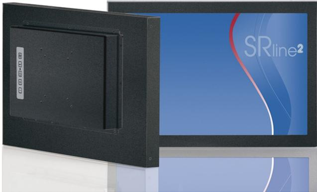
15.6" multi-touch monitor panel front IP65 analog and DVI input 12 V DC supply Phoenix contact PCAP multi-touch 10-finger attachment with clamps or VESA 75/100
